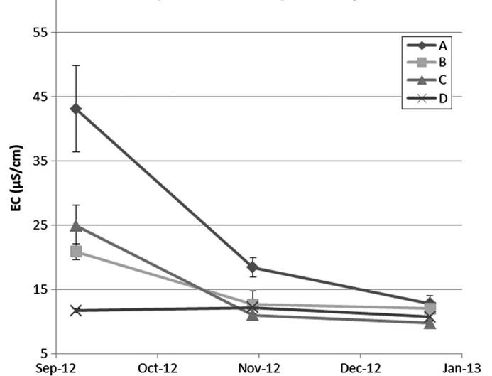
**Fig. 5.** Evolution of soil EC in ethanol extract; averages at all depths
