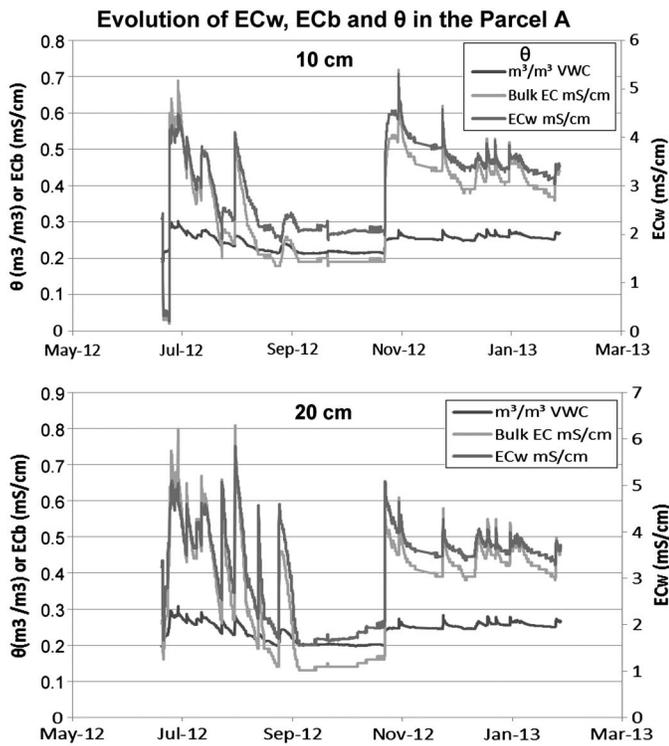
**Fig. 2.** Comparing  $EC_b$ ,  $EC_w$ , and  $\theta$  during the experimental period in parcel A at both depths
